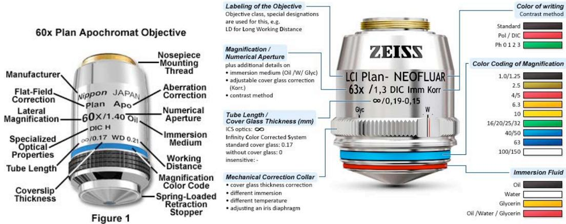
The objectives turn in the counter-clockwise direction. They go from low magnification (10X) to high mag (up to 100X). NEVER EVER EVER UNSCREW AN OBJECTIVE OUT OF ITS POSITION! they are NOT interchangeable!
